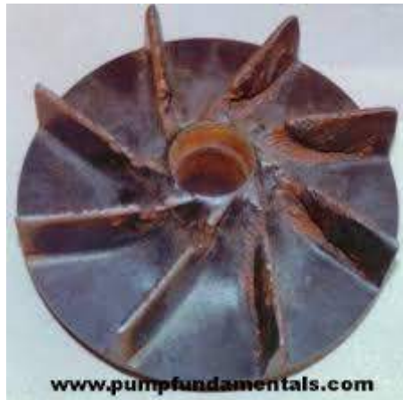
Fig.12 Cavities in pump impeller
